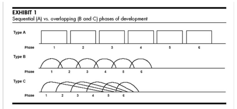
Exhibit 1 illustrates the difference between the traditional, linear approach to product development and the rugby approach. The sequential approach, labeled type A, is typified by the NASA-type PPP system. The overlap approach is represented by type B, where the overlapping occurs only at the border of adjacent phases, and type C, where the overlap extends across several phases. We observed a type B overlap at Fuji-Xerox and a type C overlap at Honda and Canon.
